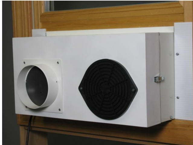
Figure 4: Hold the Fresh Air Duct Adapter up to the face of the ERV with the latches swung to the sides, then secure the latches to the strikes and close them.
