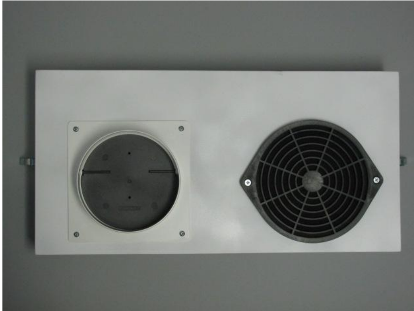
Figure 2: Attach the IQAir® "internal flange with backdraft damper" to the PuriFresh® "fresh-air duct adapter" with the #6 screws and nuts.
